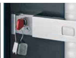
The security cylinder of LIGHTDOOR is protected against vandalism - a handle with a magnetic encoded system slides allowing key insertion.
